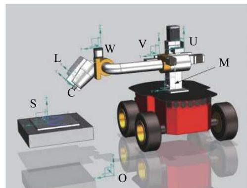
Fig. 2 Coordinate system of mobile welding robot
