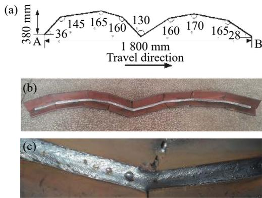
**Fig. 5 Tracking results of a complex-trajectory weld seam (a) Complex trajectory welding (b) Seam tracking test result (c) Weld detail at chamfer**
