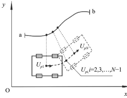
Fig. 3 Motion trajectory generation of a continuous path
