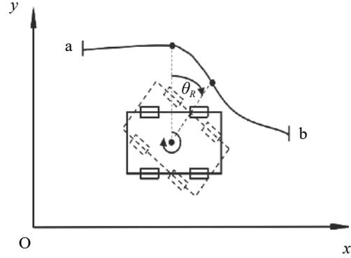
Fig. 4 Motion trajectory generation of pivot steering
