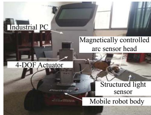
Fig. 1 Mobile welding robot system with structured light vision sensor and arc sensor
