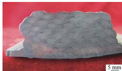
**Fig. 8 Cross section of a CMT additive manufactured component**
